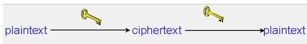
Figure 2: Secret key Cryptography. SKC uses same secret key for both encryption and decryption
